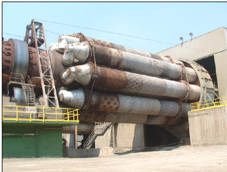
Figure 1.18: Example of a planetary cooler [45, Schorcht, 2006], [90, Hungary, 2006]
