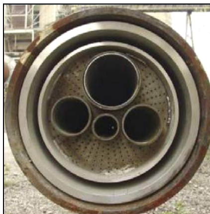
Figure 1.11: Example of a multi-channel burner [107, Belgium, 2006]
