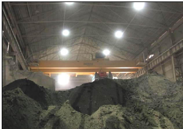
Figure 1.5: Example of covered raw material storage [81, Castle Cement UK, 2006]
