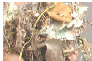
Figure 1.9: Specially prepared household waste used as fuel in cement kilns [82, CEMEX Rugby UK, 2006]
