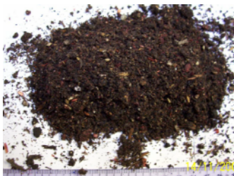
Figure 1.7: Hazardous waste – impregnated sawdust [168, TWG CLM, 2007]
