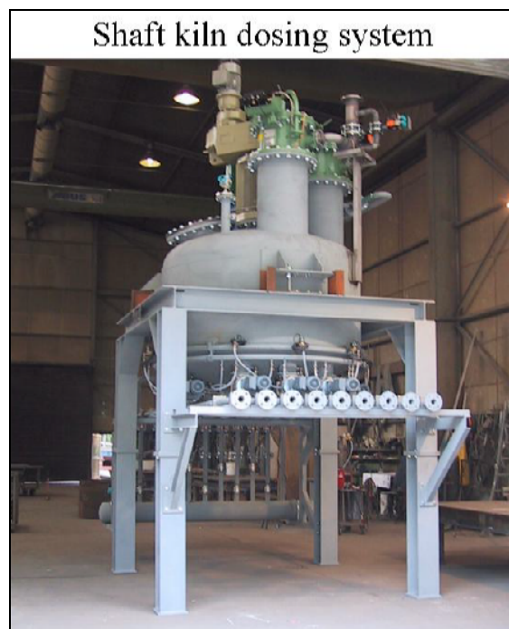
Figure 2.11: Example of a shaft kiln dosing system [44, EuLA, 2006]
