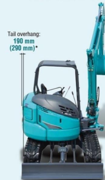
\*Figure shows the value of SK45SRX/SK55SRX with add-on counterweight.
