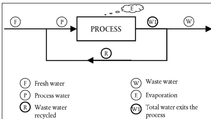
Figure A1: Water flow scheme that shall be used to calculate water recycling ratio <sup>(1)</sup>
