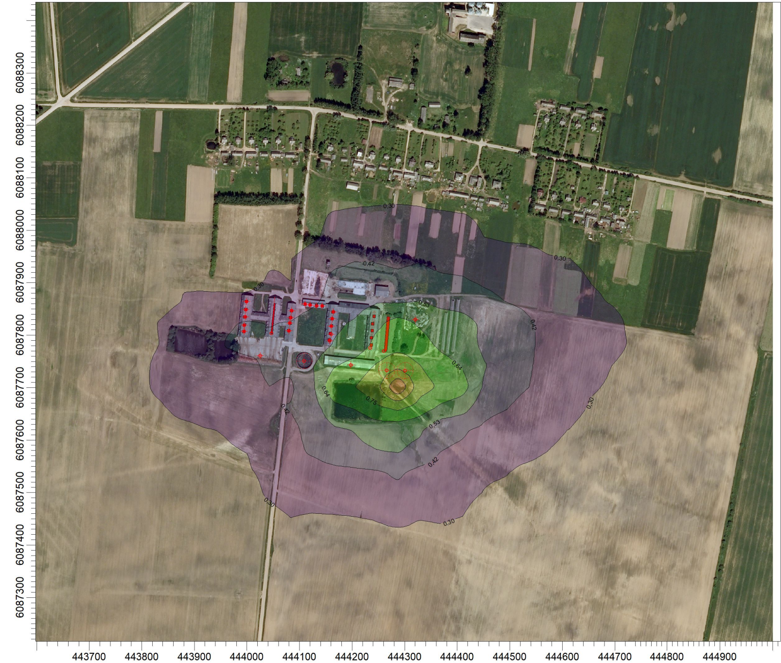
PLOT FILE OF 99.80TH PERCENTILE 1-HR VALUES FOR SOURCE GROUP: NO2 Max: 1,09 [ug/m^3] at (444285,18, 6087703,12)
