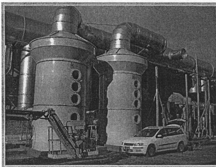
Fig. 2: indicative picture of Ecochimica floating scrubbers
